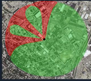
Nearby antennas "shade" or "notch" the desired omni-directional antenna pattern leading to unpredictable coverage holes.
